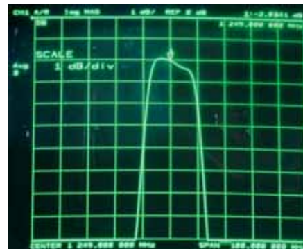
23cm filter close-in response, 1dB/div, centre 1249MHz, span 100MHz
